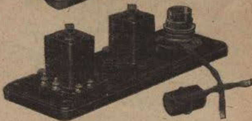
Showing the Relay of the Remote Control for set using L.T. Accumulator and H.T. Eliminator.
